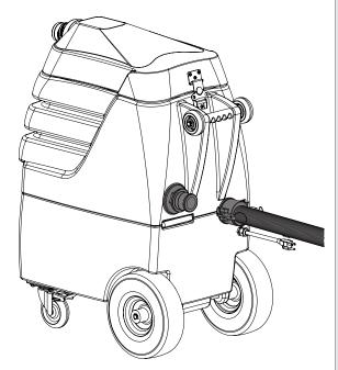
Attach the second hose bearing cam lock to the Auto Pump-out fitting. Secure the hose to the fitting using the cam lock. Push the hose cuff onto the fitting, making sure the silver ears and rings are extended forward. Pull the ears down using the rings until connection is tight. Place the end of the hose in a location where dirty water can drain.
