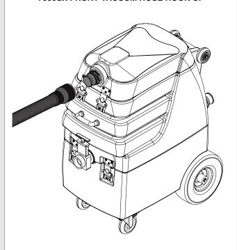
Attach the hose with the 1.5" Cuff-Lynx™ reducer to the machine. Attach other end of same hose to wand tube.
